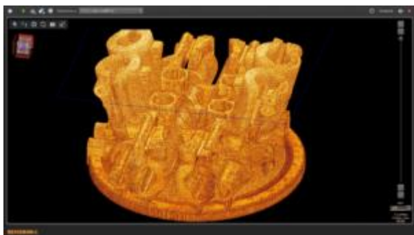
Figure 15 Renishaw InfiniAM Spectral software for laser powder-bed fusion (LPBF) technologies
