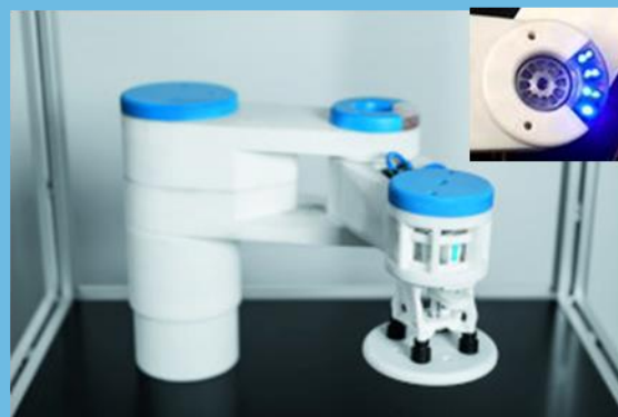
Fully printed electronic parts embedded in printed robotic arm
